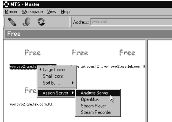
Figure 2-21: Port Manager panel showing Analysis Server selected
